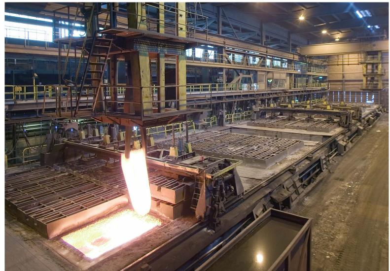
48 furnaces converted to oxyfuel combustion at Ovako Steel, Horfors works, Sweden
