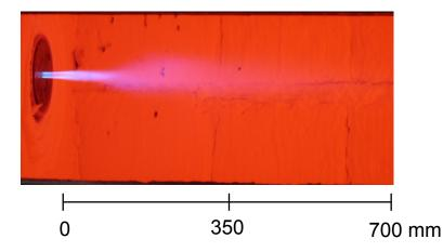
oxyfuel staged combustion with 5 % primary oxygen
