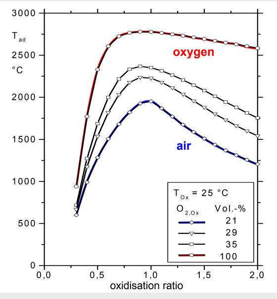
theoretical adiabatic combustion temperature using high calorific natural gas and different oxidators
