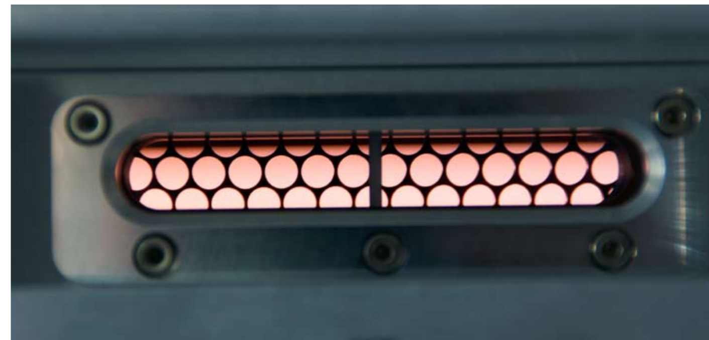
F_2 plasma as seen from the PECVD tool chamber window
